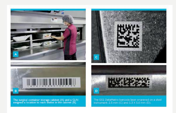
The hospital's surgical container storage cabinet (A) and a GLN assigned a location to each shelve in the cabinet (B). The GS1 DataMatrix barcode laser engraved on a steel instrument: 2.5 mm X 2.5 mm (C) and 1.3 X 5.0 mm (D).
