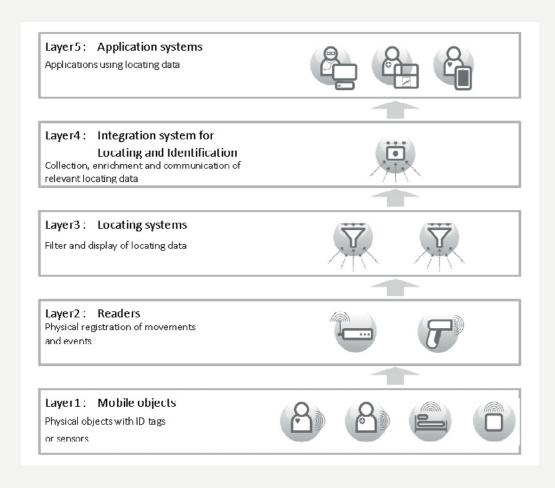
By layering the architecture, the model supports multiple tracking technologies that can be replaced at any time without affecting the business applications subscribing to the tracking data.
